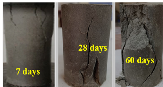
Figure 8. Crack patterns observed in SM2NH12 specimens at 7 days, 28 days, and 60 days.
