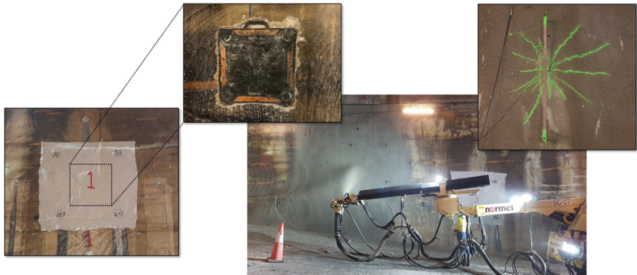
Figure 5. Photos of the large-scale field testing on shotcrete lining.
