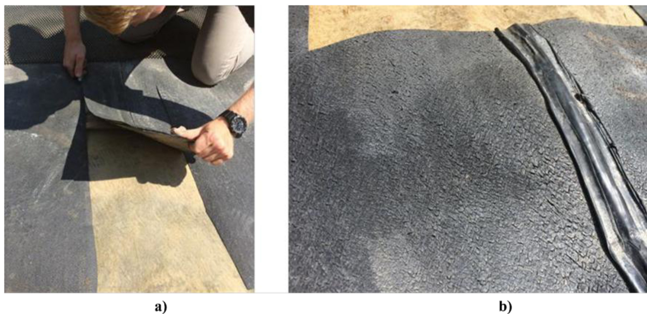
Figure 4. Field exhumation procedures conducted by Rafter et al. (2018): (a) extraction of HDPE geomembrane sheet samples; (b) sampling of extrusion welds.
