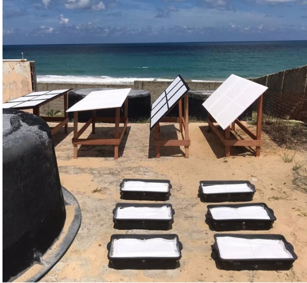
Figure 1. Field test in operation with tables inclined at 45° and sandboxes inclined at 0°.
