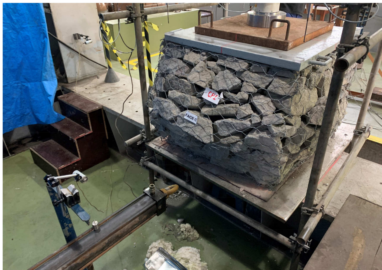
Figure 4. Deformation of the box with hexagonal mesh (Type A). Note the difference in relation to the Type C box, in Figure 5.
