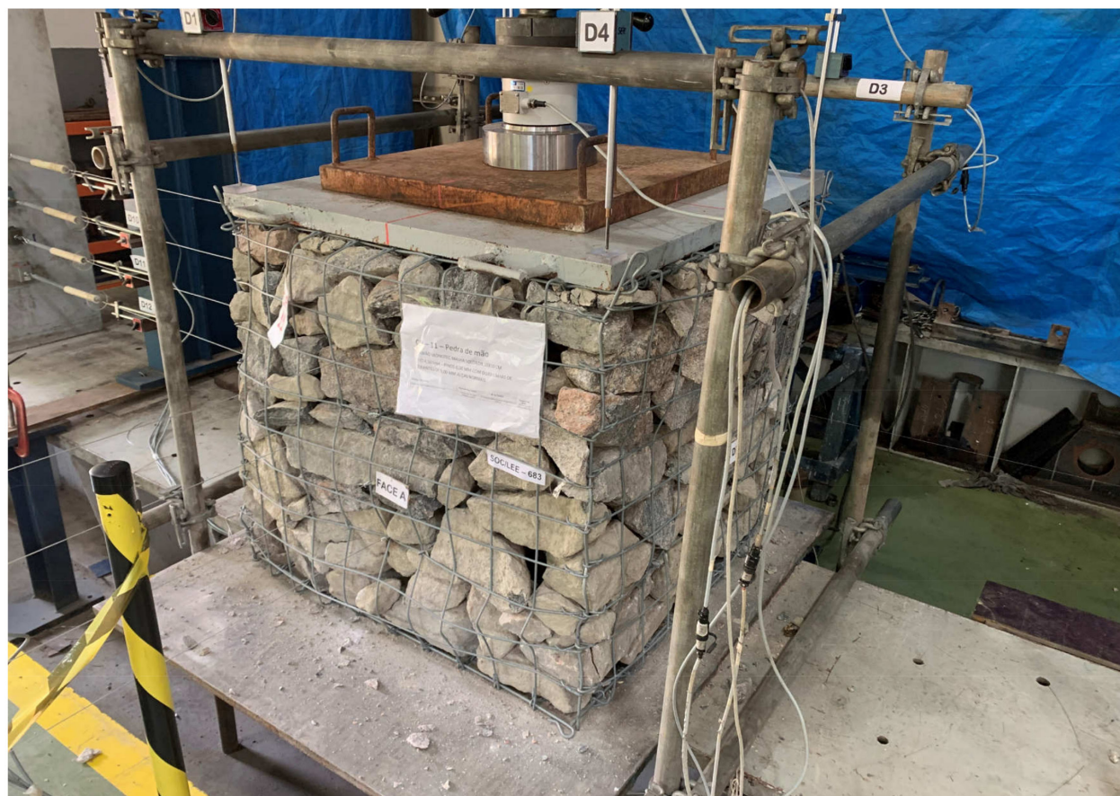
Figure 2. Apparatus used in unconfined tests.
