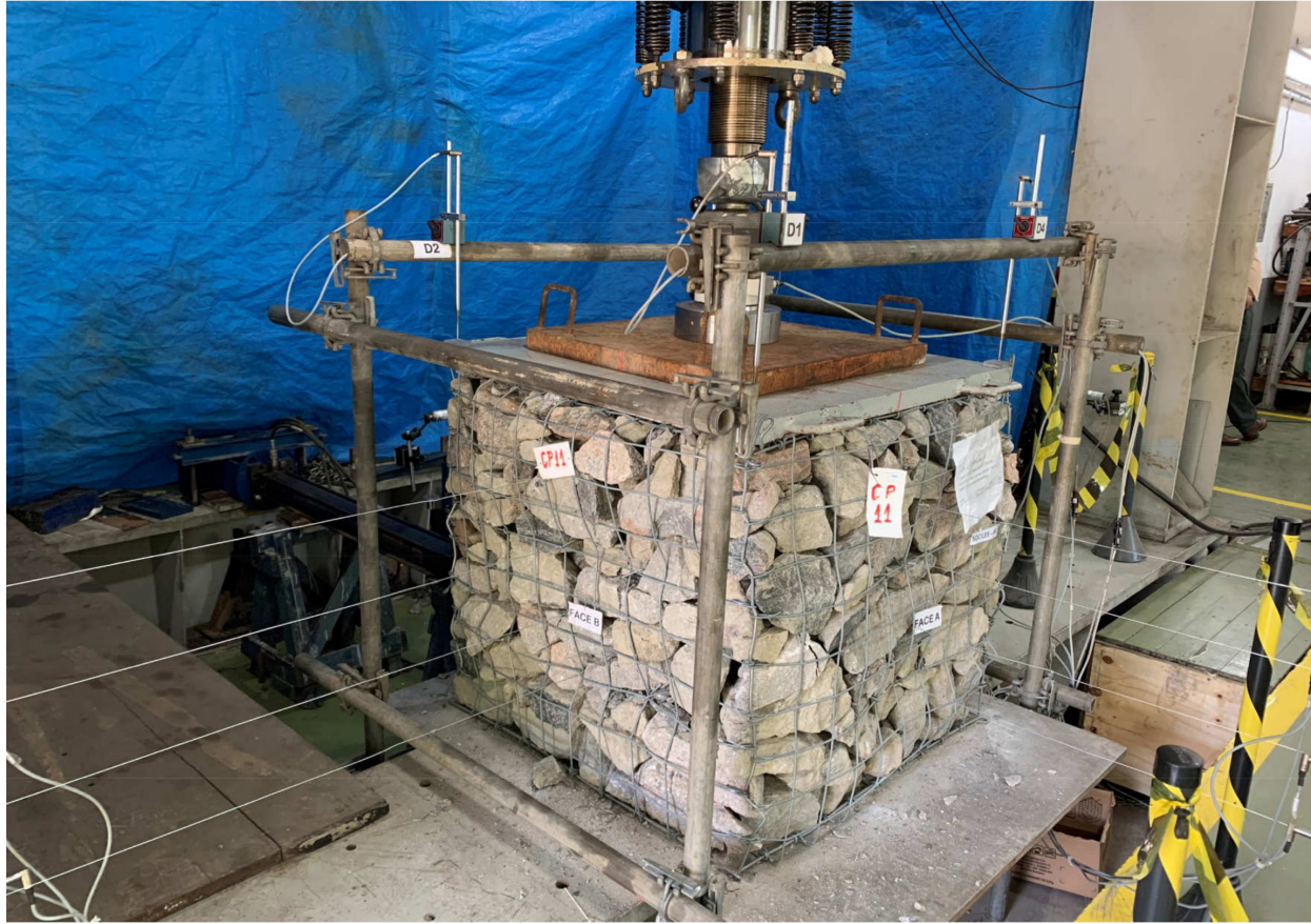
Figure 5. Deformation of the box with coated carbon steel mesh and connection pins (Type C).
