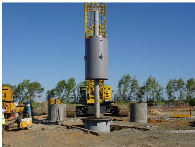
Figure 1. SIPEX: Drop mass system 100+100 kN.
