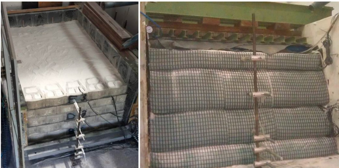
Figure 15. Views of a block and wrapped-face walls.
