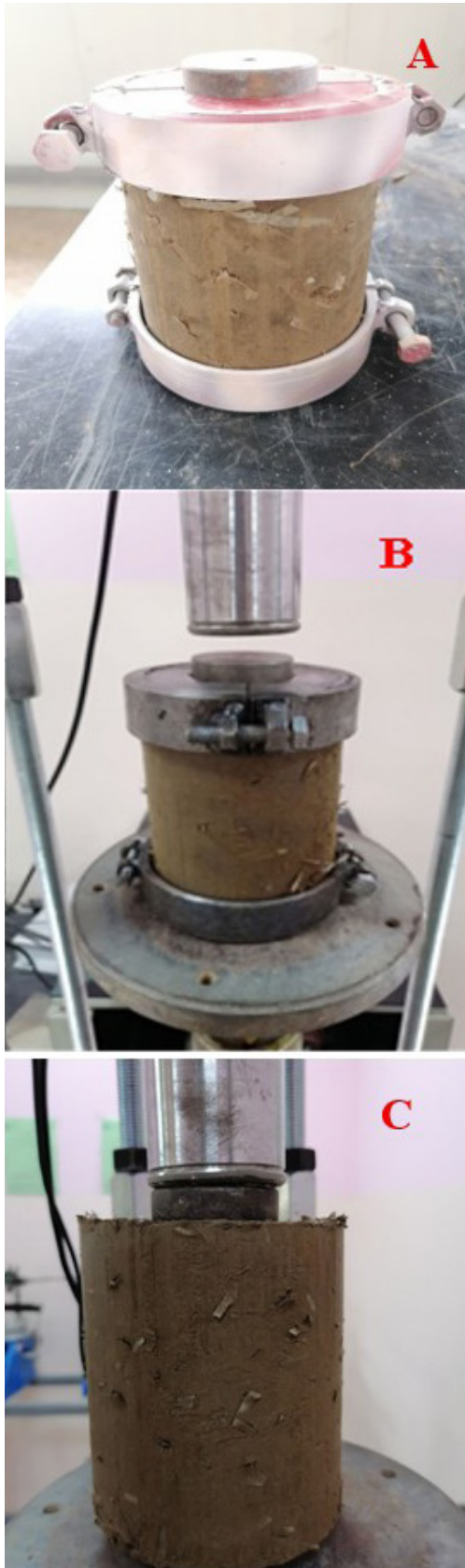
Figure 2. Punching test: (A) sample with metal rings to align loading discs; (B) fixing the sample for test; (C) sample under testing.
