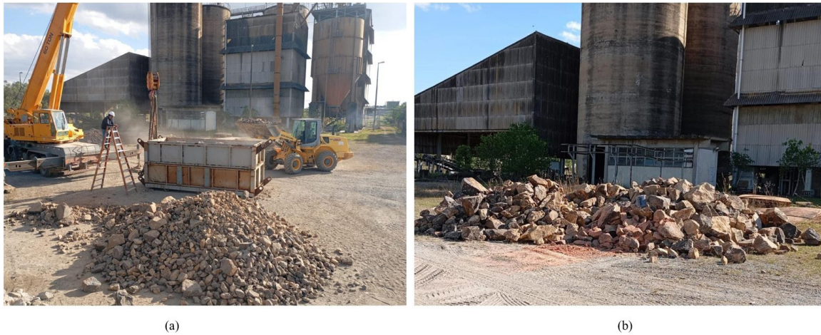
Figure 2. Grain size distribution of the rip rap: (a) D_{50} = 150 mm; (b) D_{50} = 600 mm.
