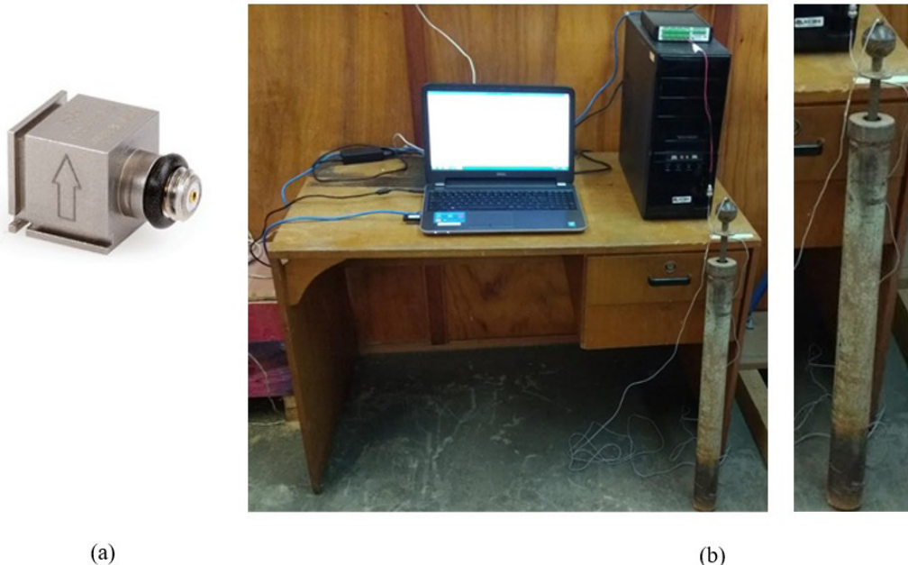
Figure 1. Damping Ratio ( D ) Measurement Equipment: (a) Bruel & Kjaer 4507-B-005 Piezoelectric IEPE accelerometer; (b) Schematic figure of the apparatus for damping ratio measurements.
