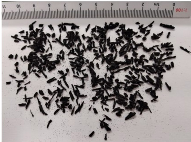
Figure 4. Rubber chippings employed in this research were obtained from shredded scrap tires (scale in centimeters).
