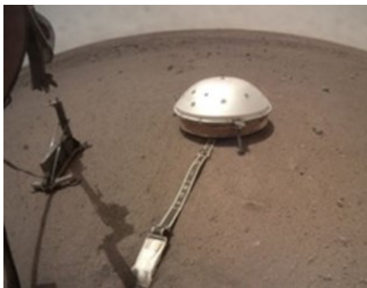
Figure 3. Image taken from the Instrument Context Camera (ICC) on sol 87 (local time 11:54:07 LMS) showing the location of SEIS and of the HP 3 support structure, 1.18 metre apart from each other (image credit: JPL/NASA).
