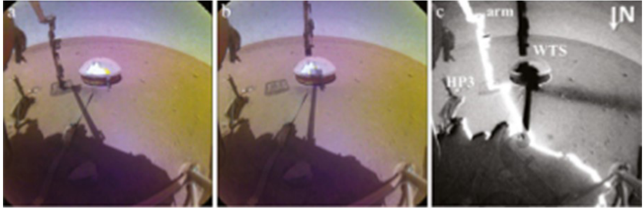
Figure 30. (a) Instrument Context Camera (ICC) image taken on sol 877 at 11:22 a.m. before dump 6 on the SEIS tether; (b) ICC image acquired on sol 877 at 11:33 a.m., after dump 6; (c) ICC image difference showing the dark plume made up of wind dispersed and transported particles. The plume extends to the right from the WTS, and its orientation corresponds to the wind direction from N14° (ESE) to N320° (WNW) (Verdier et al., 2023).
