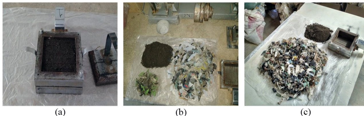
Figure 2. Molding process for solid waste specimens: (a) 100% basic matrix; (b) 83.83% basic matrix + 16.17% fibers; and (c) 67.67% basic matrix + 32.33% fibers.
