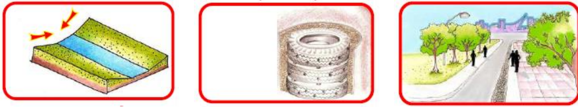
Figure 1. Infiltration structures (modified from Lelis & Camapum de Carvalho, 2011).
