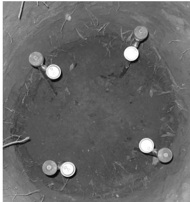
Figure 11 - Tensiometers positions in the control pit.
