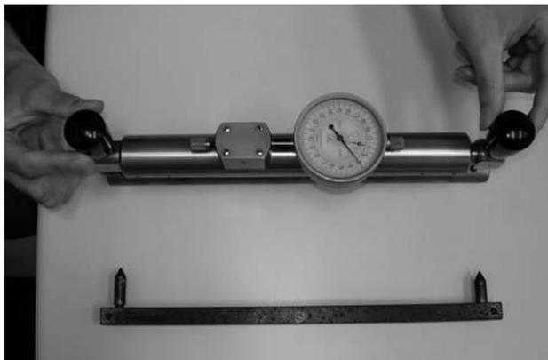
Figure 4 - Mechanical extensometer Huggenberg used to measure the strains in the columns.
