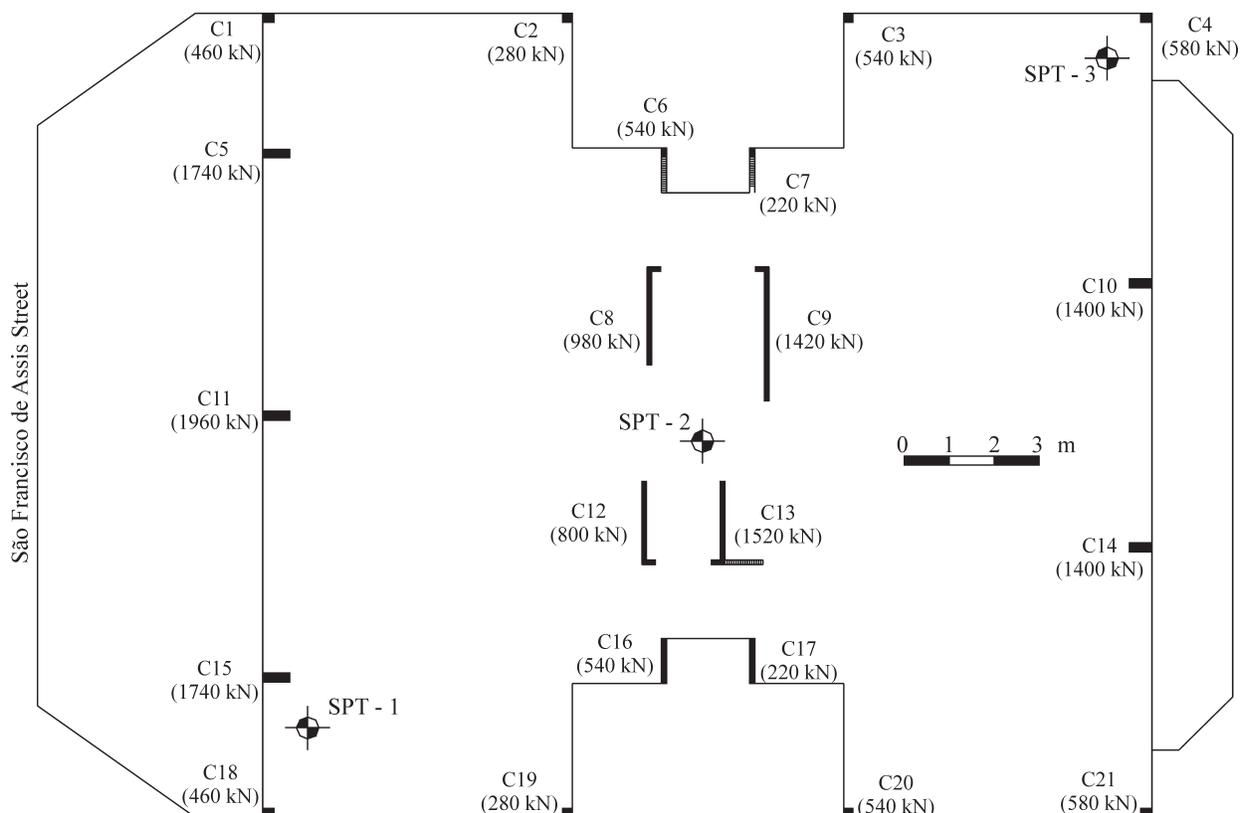
Figure 2 - Location of columns and SPT's performed (Gonçalves *et al.*, 2004).
