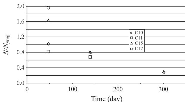
**Figure 10** - Ratio between the column loads obtained from the measured strains and the loads from the finite element analysis versus time (Gonçalves, 2004).
