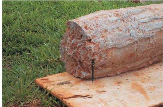
**Figure 6** - Exhumed testing CFA pile.
