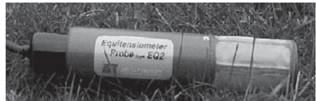
Figure 8 - Equitensiometer (EQ2) [Delta - T Devices].
