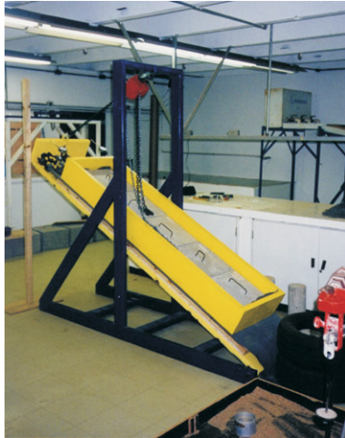
Figure 5 - Large scale ramp test equipment.
