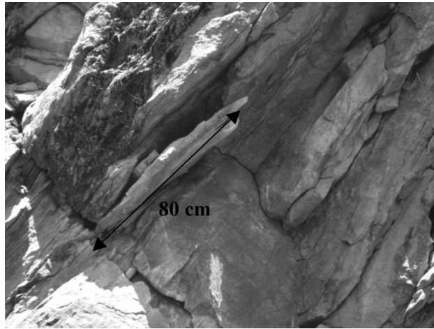
Figure 6 - Format of block in ES-166 (2) slope.
