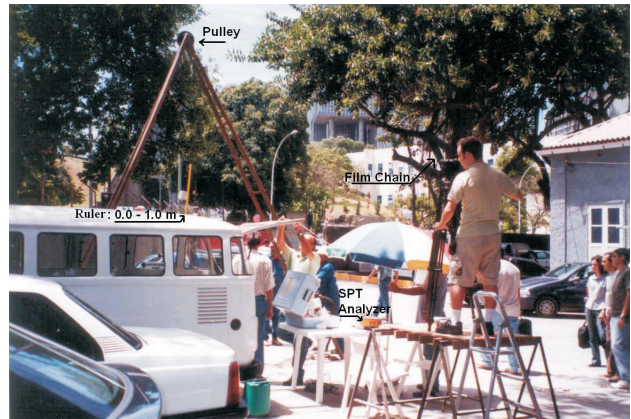
Figure 12 - System used to evaluate drop height, impact velocity and energy below the anvil.
