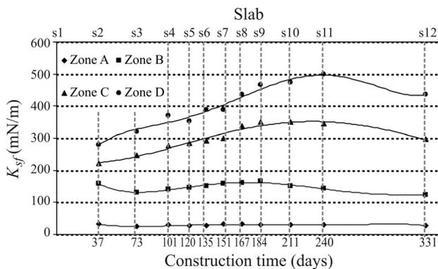
Figure 12 - Curves of average values of  $K_{sf}$  coefficient for zones SFA, SFB, SFC and SFD during construction.
