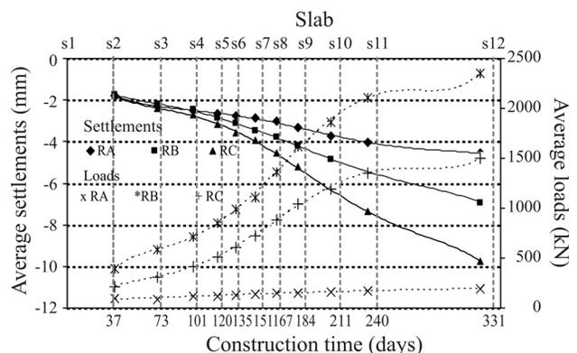
Figure 16 - Evaluation of mean settlement and loads during construction.
