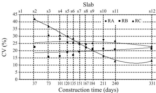
Figure 18 - Evolution of the settlement variation coefficients for regions RA, RB and RC over time of construction.
