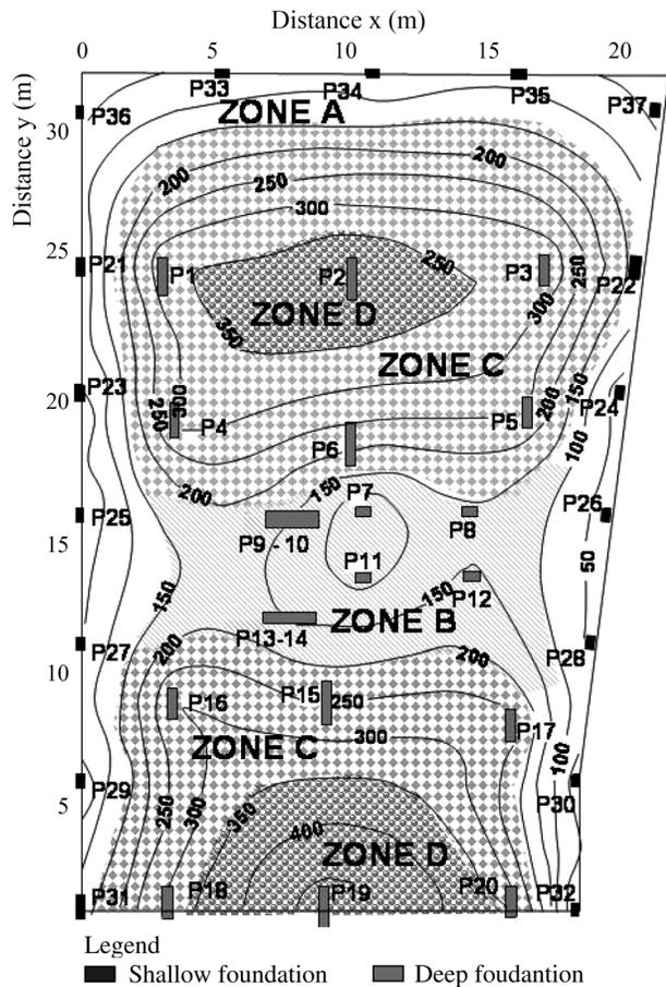
Figure 11 - Contours of  $K_{sf}$  for the last stage of construction (MN/m).
