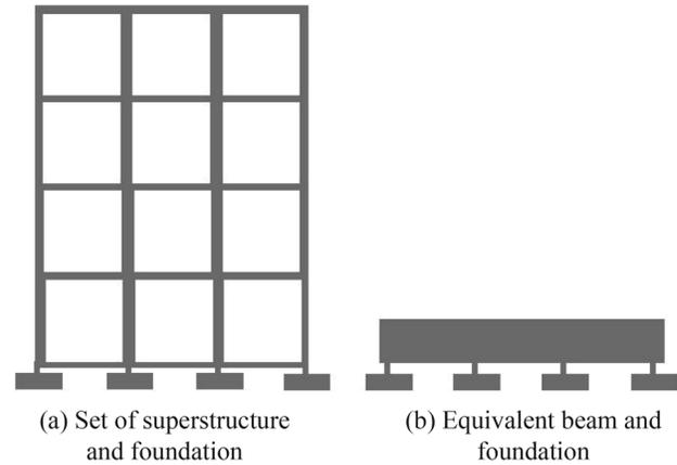
**Figure 4** - Beam with equivalent stiffness proposed by Meyerhof (1953).
