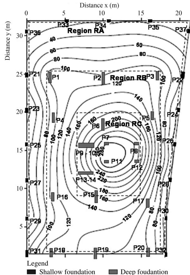
Figure 13 - Contours of equivalent coefficient curves ( $K_e$ ) for the last stage of construction (MN/m).
