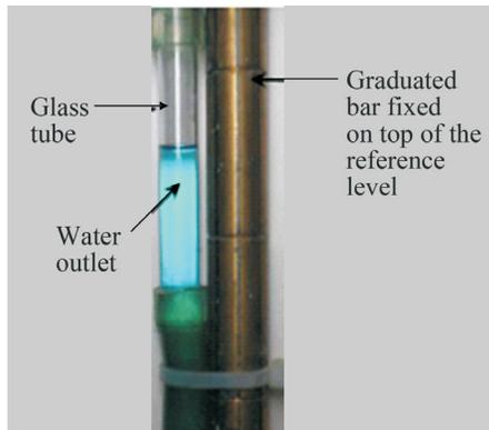
**Figure 8** - Metal post and water outlet on the reference mark.
