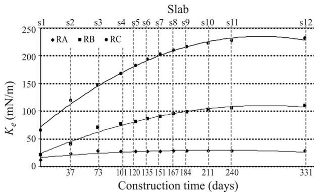
Figure 14 - Variation of the equivalent stiffness coefficient ( $K_e$ ) for regions RA, RB and RC during construction.
