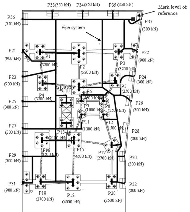
Figure 7 - Sketches of the foundations, location of columns with respective design loads, level reference mark, pipe network and project loads.
