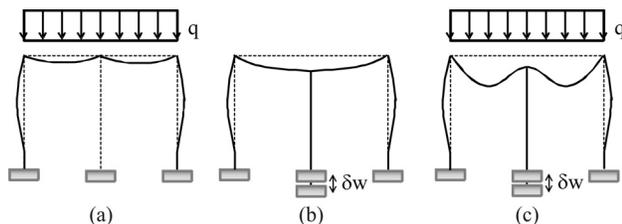
Figure 1 - Soil-structure interaction model.
