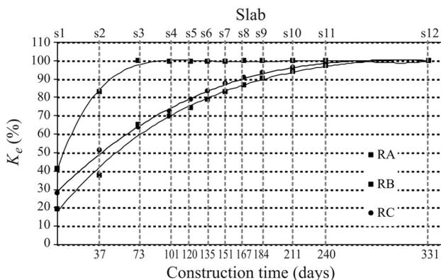
Figure 15 - Proportional evolution of the equivalent stiffness coefficient ( $K_e$ ) of the structure for regions RA, RB and RC.
