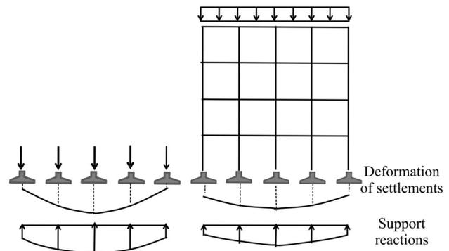
Figure 2 - Effect of SSI on settlements and support reactions (adapted from Gusmão (1994)).
