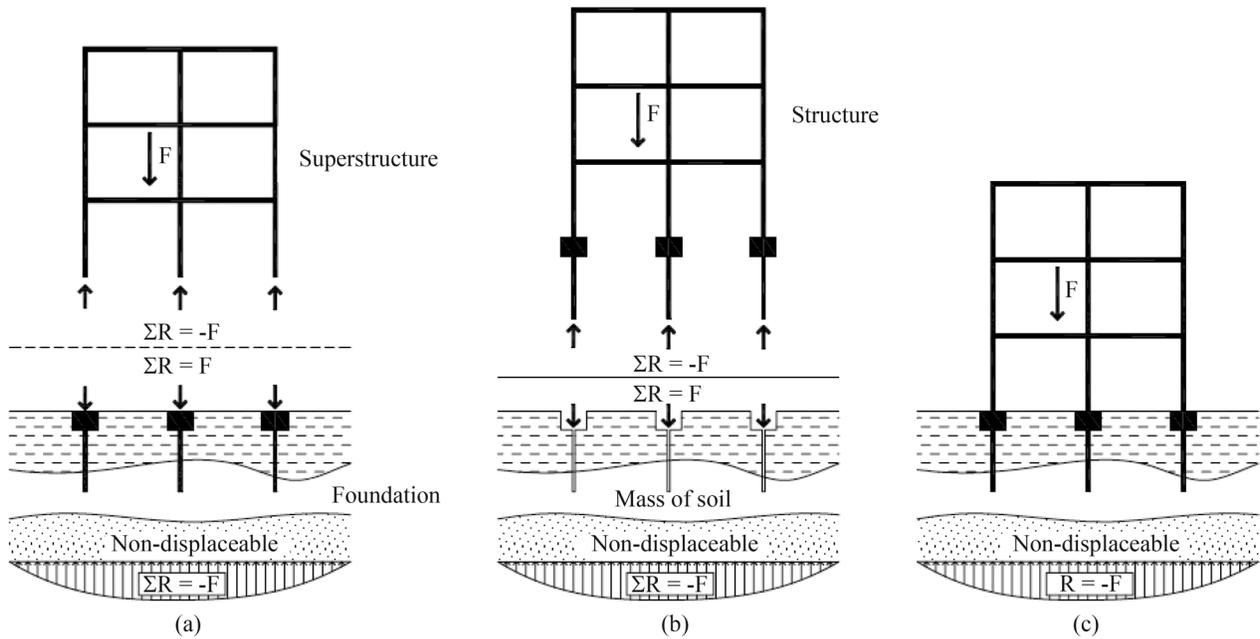
Figure 5 - Models for soil-structure interaction analysis (adapted from Mota *et al.*, 2007).
