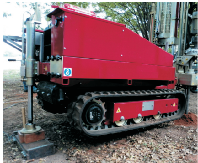
Figure 8 - Photo of the seismic source placed in the rear of the pushing equipment.
