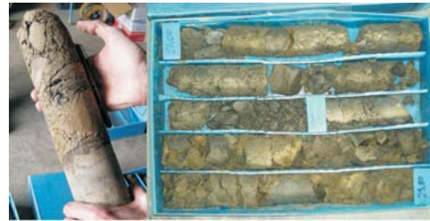
Figure 6 - Borehole cores of the calcareous breccias of the slided material.
