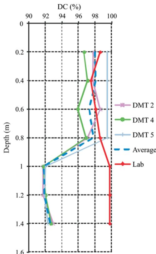
**Figure 7** - Degree of compaction.
