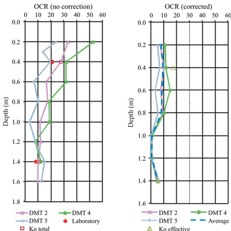
Figure 4 - OCR values calculated with and without the effect of suction.
