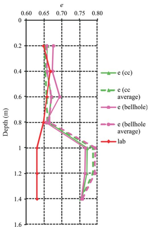
**Figure 6** - Void ratios obtained for different soil moisture conditions.
