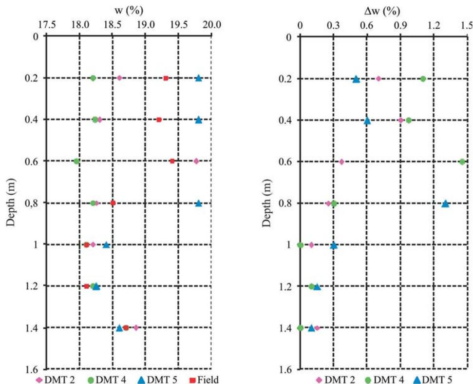
**Figure 5** - Moisture values obtained in the laboratory and those found using the characteristic curve, and deviations of moisture (in module)
