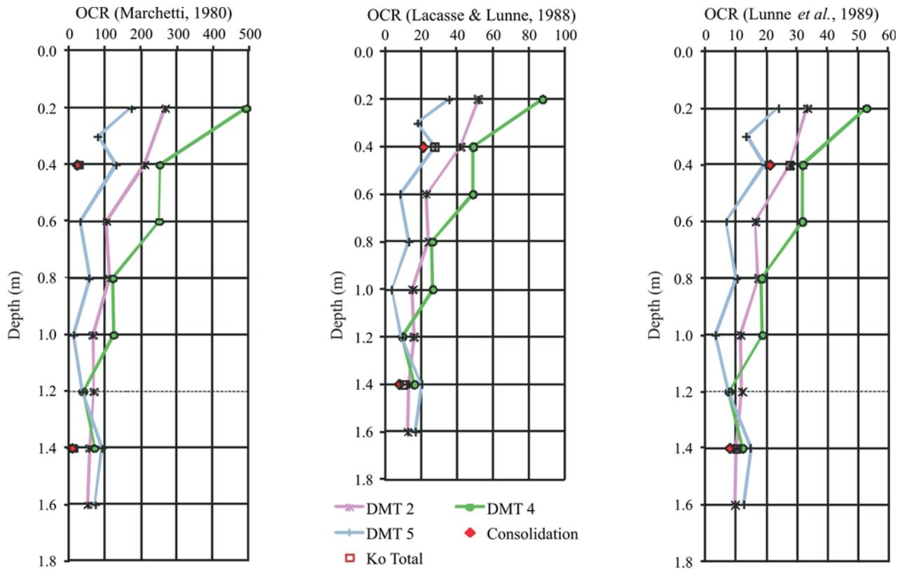
Figure 2 - OCR calculated from oedometric compression testing and DMT.
