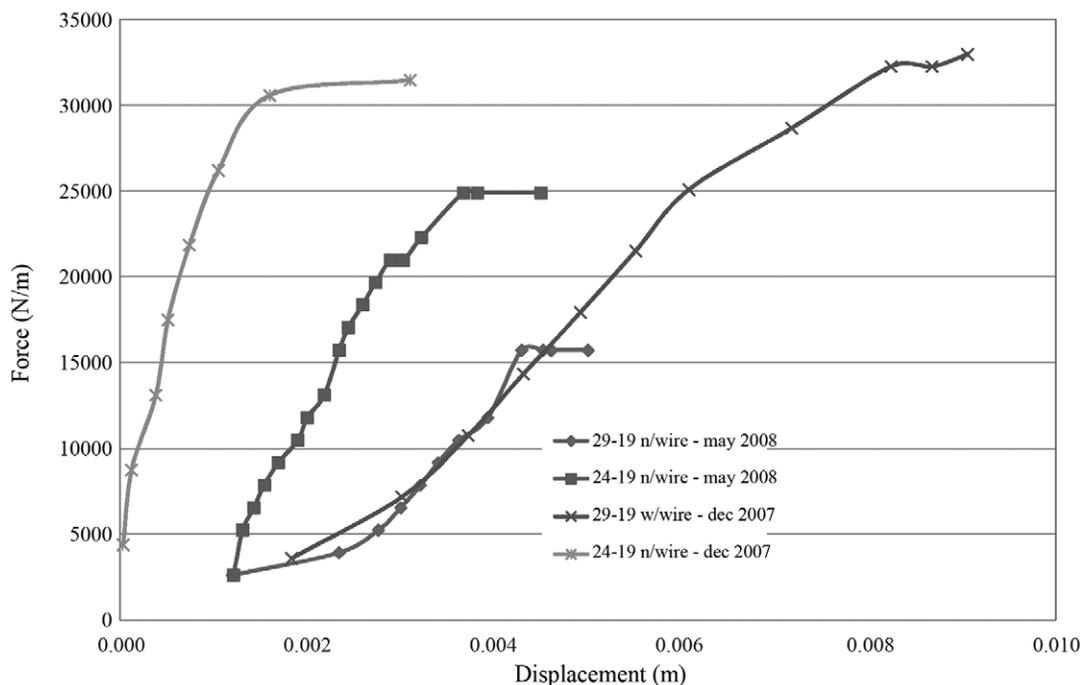
**Figure 4** - Force/displacement for pullout tests.
