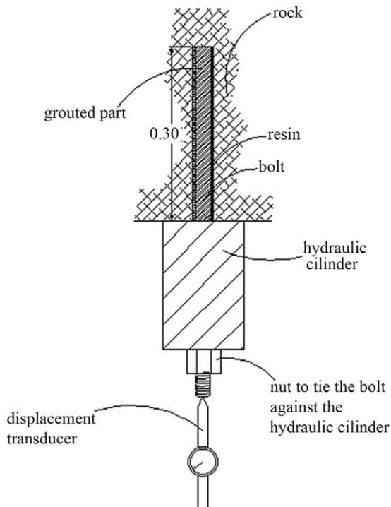
**Figure 3** - Apparatus for pullout test.
