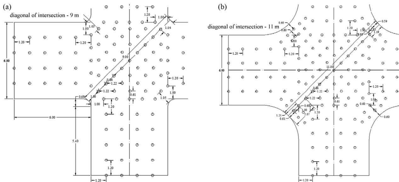
Figure 6 - New roof support design for intersection, considering 1.8 m long roof bolt for diagonal (a) 9 m, and (b) 11 m.
