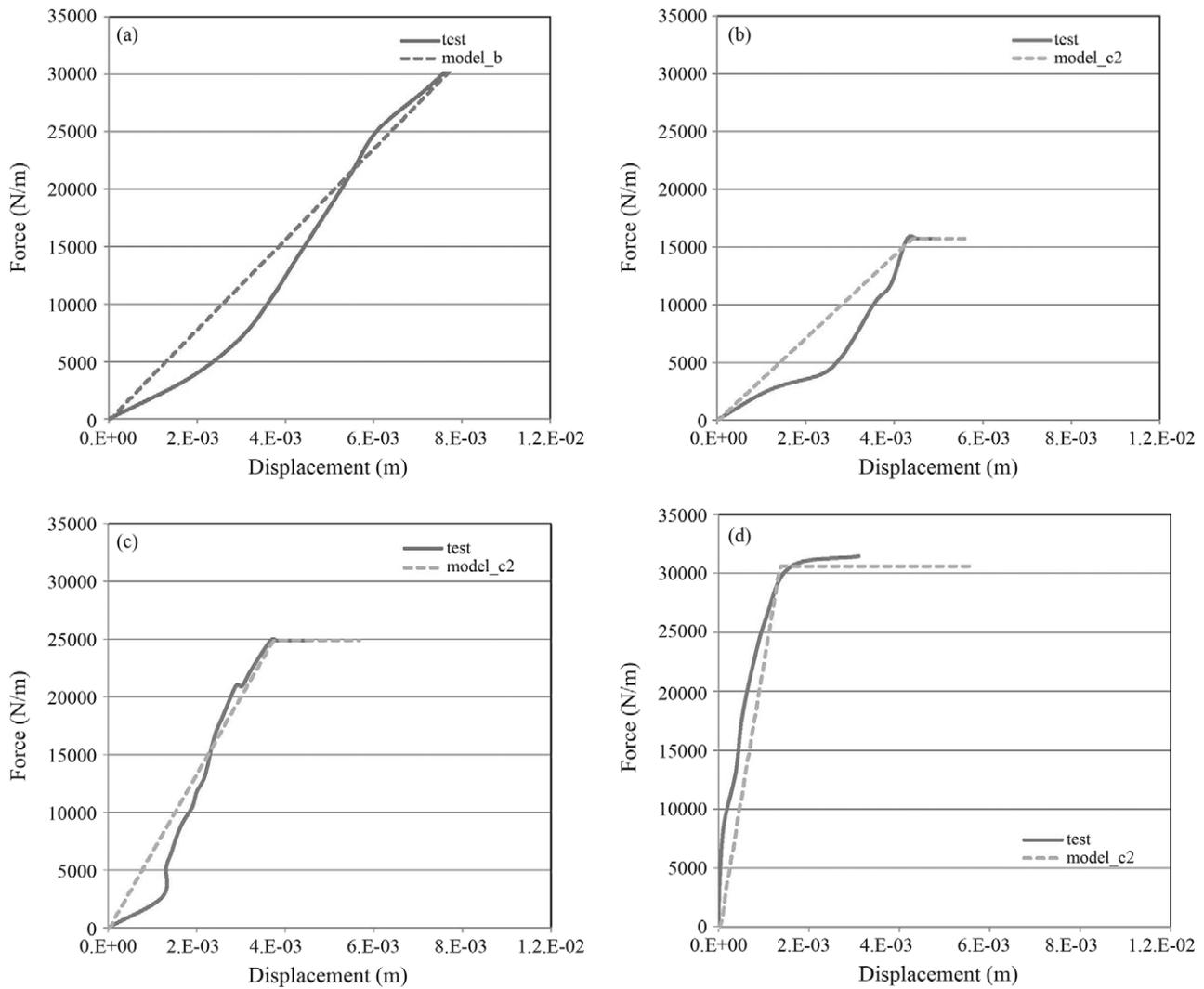
**Figure 5** - Results of the numerical simulation for pullout tests compared to the field tests. (a) Borehole 29 mm and bolt with steel wire; (b) Borehole 29 mm and bolt with no steel wire; (c) and (d) Borehole 24 mm and bolt with no steel wire.
