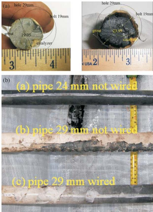
**Figure 2** - (a) picture of the cross-section of a resin cartridge, and (b) results for grout mixture tests.
