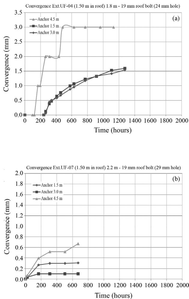
Figure 7 - Roof convergence for (a) new roof support design, and (b) old roof support design.
