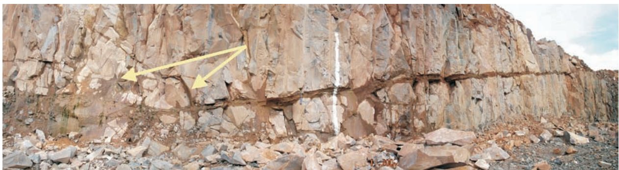
Figure 7 - “Fault-joints” in basalts of Northern Brazil. Observe ramifications on the left end. The photo was taken during dam construction.
