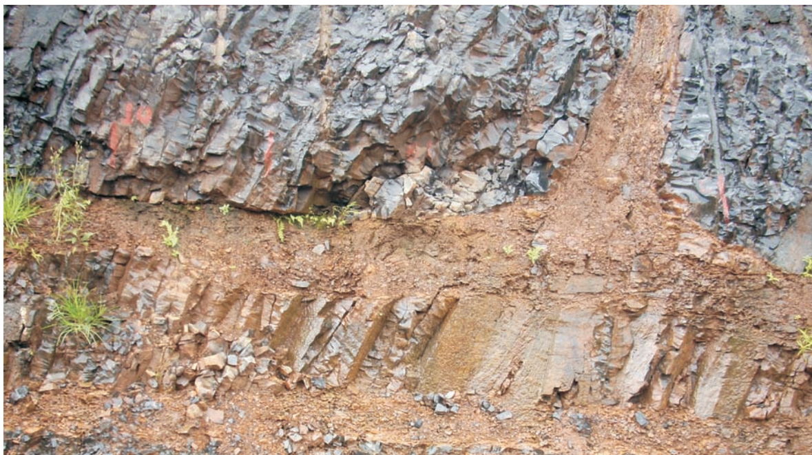
Figure 8 - Weathered “Fault-joint” between colonnade and entablature (upper realm) at a dam construction site in Parana Basin basalt flow in the São Paulo State.
