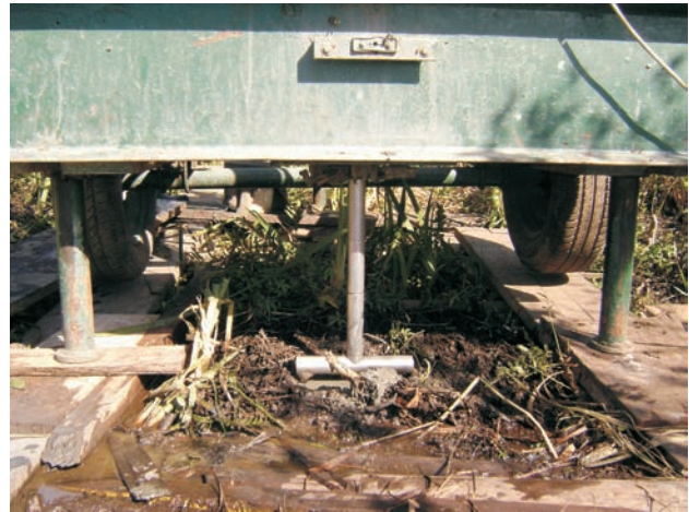
Figure 14 - T-bar in the beginning of a test at Sarapuí II test site, where the intense presence of roots can be noted.
