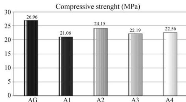
**Figure 8** - Compressive strength of the concrete at 28 days of age (MPa).
