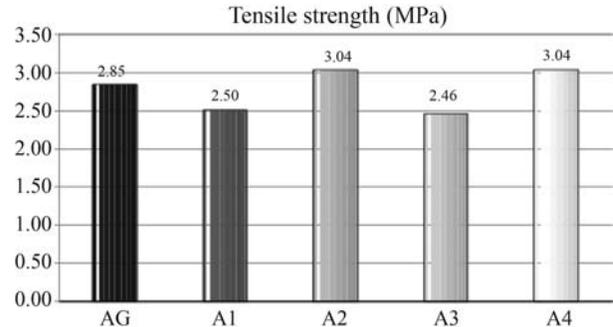
**Figure 11** - Tensile strength by diametral compression of aggregates on the 28<sup>th</sup> day.
