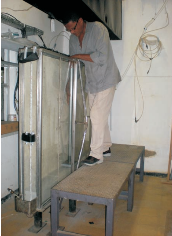
Figure 3 - View of the flow channel with sand compaction in progress. Features: steel bar lattice to reinforce the channel structure; back wall coated with epoxy & sand; sidewall reservoir to hold the Mariotte tube.
