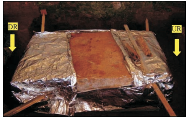
Figure 6 - Excavation of the upstream (UR) and downstream (DR) reservoirs.
