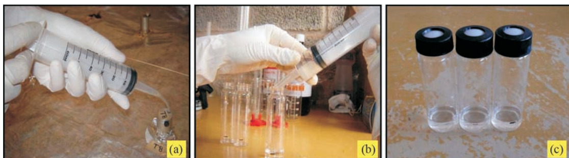
Figure 13 - (a) Introduction of the hose in the monitoring tube; (b) Injection of the contaminated solution in the vial; (c) Sealed vials.
