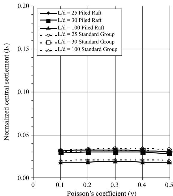
**Figure 3** - Effect of the variation of some initial parameters on the settlement value.
