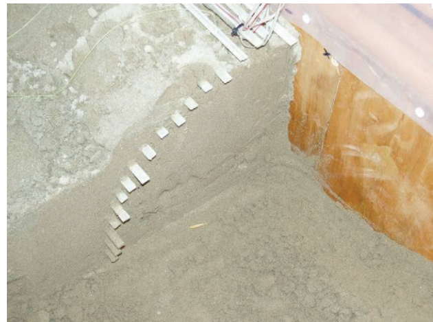
Figure 2 - Photograph of the test box where the position of the half-tunnel and holes for reinforcing elements can be observed.
