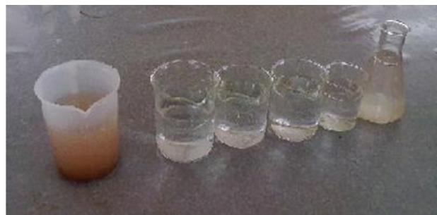
Figure 4 - The sample of the discharged water from pinhole test for dispersive and non dispersive soils.
