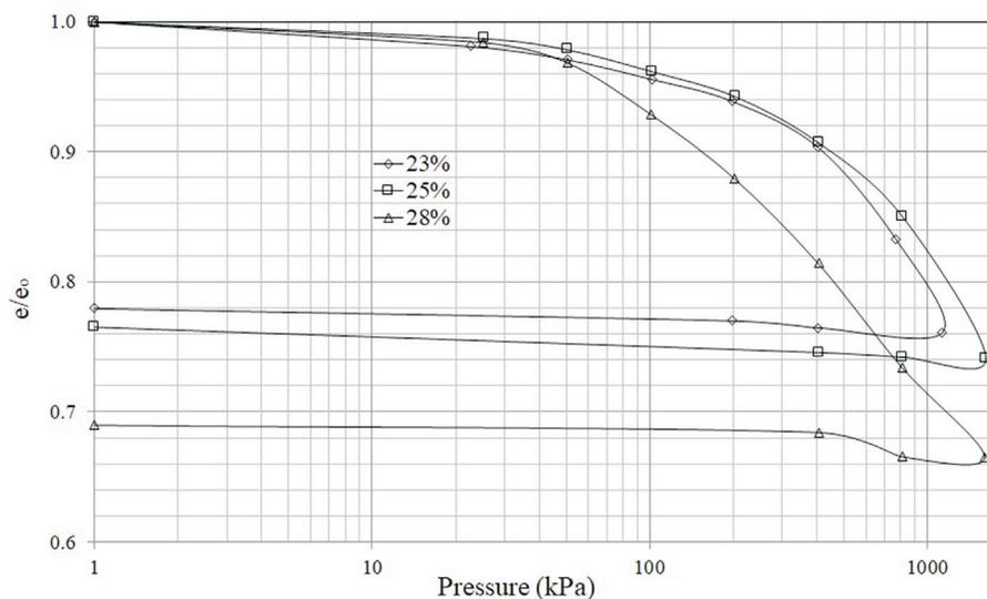
**Figure 5.** Normalized compressibility curve for the three compaction moisture contents.
