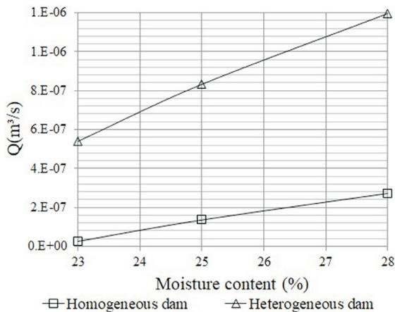
Figure 15. Flow for different compaction moisture contents.
