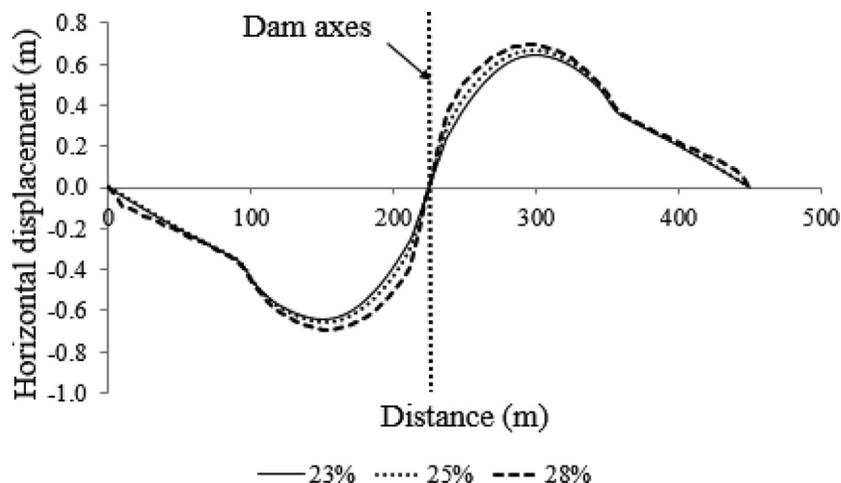
Figure 29. Maximum horizontal deformations along the heterogeneous dam.
