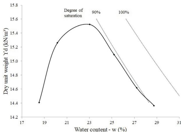
**Figure 1.** Compaction curve for the UnB experimental site soil.
