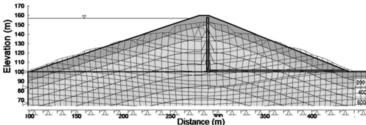
Figure 22. Total stress for the homogeneous dam.
