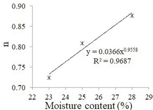
**Figure 11.** The relation between  $n$  and the compaction moisture content.
