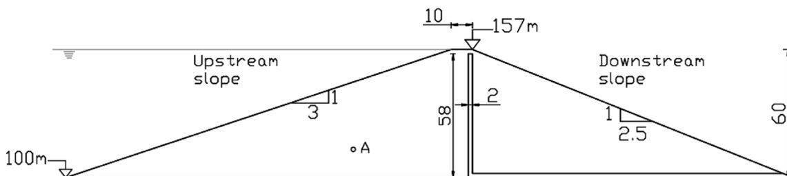
**Figure 13.** Typical cross-section 1 (homogeneous dam).
