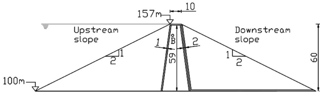
Figure 14. Typical cross-section 2 (heterogeneous dam).
