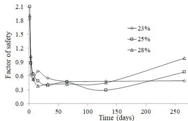
**Figure 18.** Time variation of the safety factors for the homogeneous dam.
