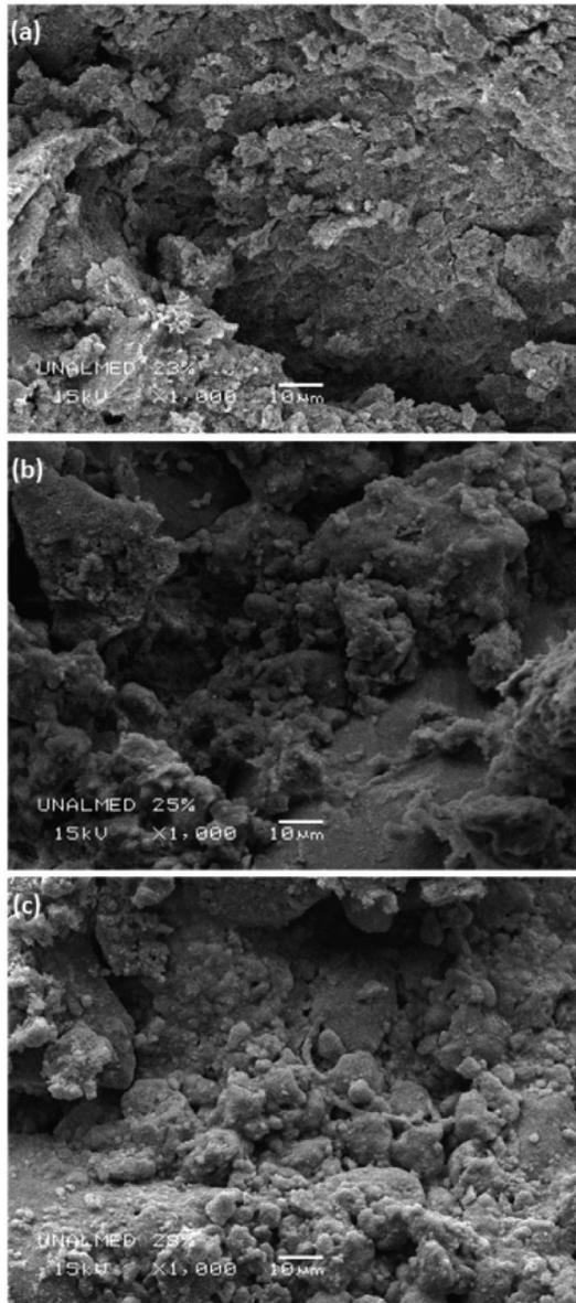
**Figure 3.** Images obtained by SEM for x1000 magnification: (a) Image of compacted soil with 23 % moisture content; (b) Image of compacted soil with 25 % moisture content; (c) Image of compacted soil with 28 % moisture content.
