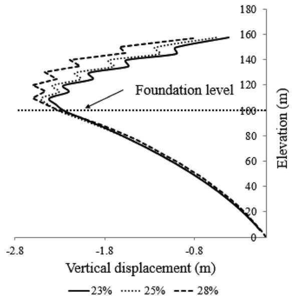
Figure 26. Maximum vertical settlement in the central axis (elevation) for the homogeneous dam.
