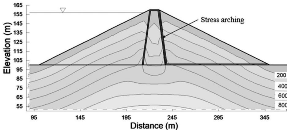
Figure 24. Total stress for the heterogeneous dam.
