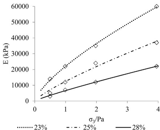
**Figure 10.** The relation between the deformability modulus and the confinement pressure.
