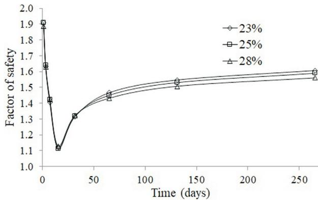
**Figure 19.** Time variation of the safety factors for the heterogeneous dam.
