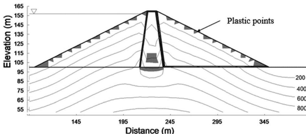
Figure 25. Plastic points for the heterogeneous dam.
