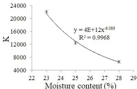
**Figure 12.** The relation between  $K$  and the compaction moisture content.
