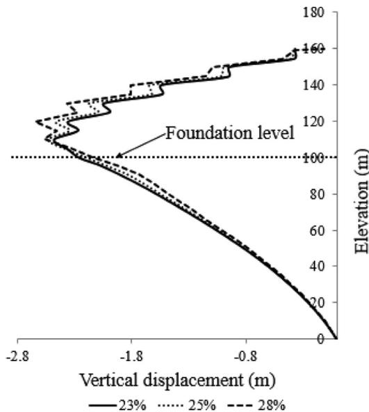
Figure 28. Maximum vertical settling in the central axis for the heterogeneous dam.
