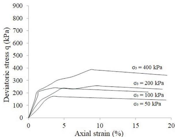
Figure 8. CID triaxial tests result for soil sample compacted at optimum moisture content +5 %.
