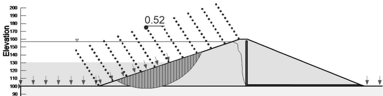
**Figure 20.** Minimum safety factor for the homogeneous dam (7-15 days - end of the rapid drawdown).
