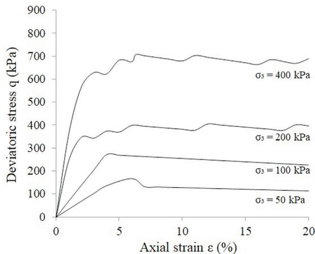
Figure 7. CID triaxial tests result for soil sample compacted at optimum moisture content +2 %.
