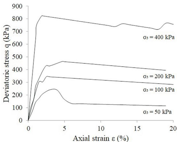
Figure 6. CID triaxial tests result for soil sample compacted at optimum moisture content.
