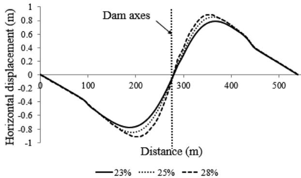
Figure 27. Maximum horizontal displacement along the homogeneous dam base.
