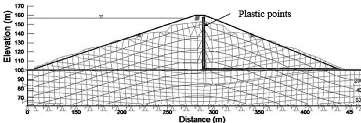
Figure 23. Plastic points for the homogeneous dam.
