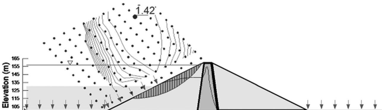
**Figure 21.** Minimum safety factor for the heterogeneous (7-15 days - end of the rapid drawdown).
