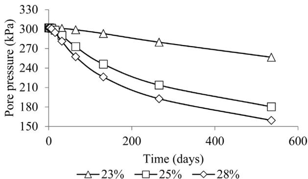
Figure 16. Pore pressures in point A for the three compaction moisture contents, homogeneous dam.
