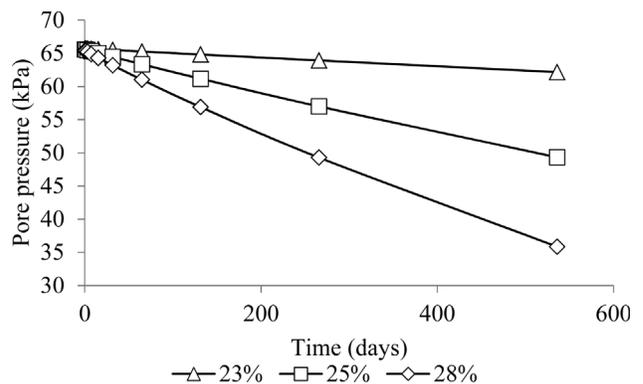
Figure 17. Pore pressures in point B for the three compaction moisture contents, heterogeneous dam.
