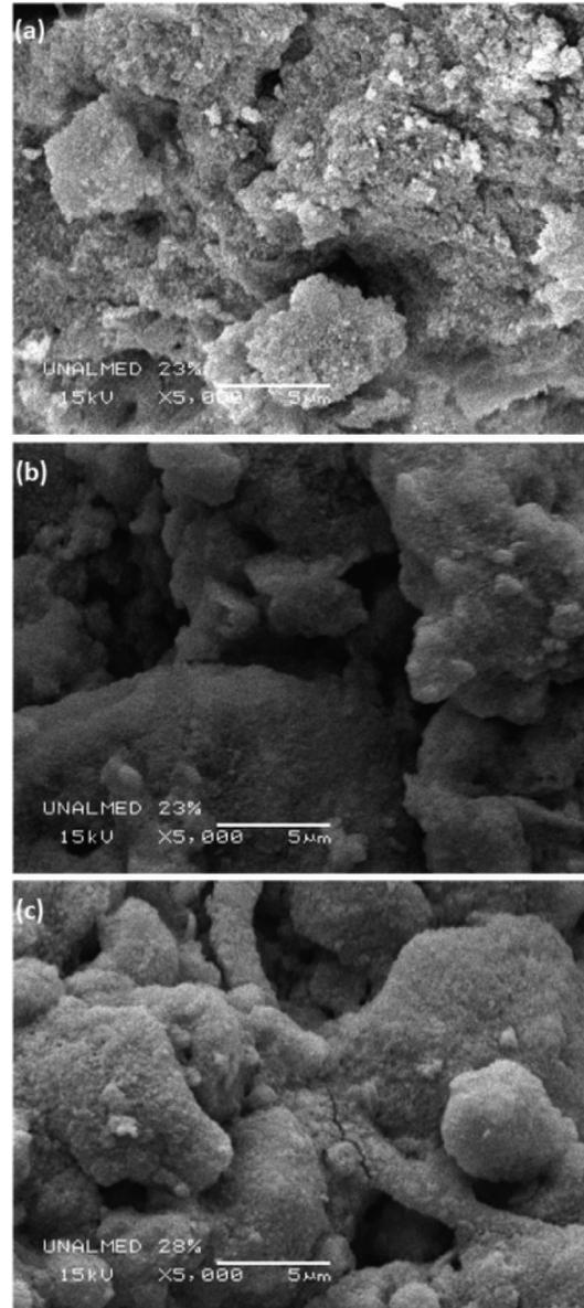
**Figure 4.** Images obtained by SEM for x5000 magnification: (a) Image of compacted soil with 23 % moisture content; (b) Image of compacted soil with 25 % moisture content; (c) Image of compacted soil with 28 % moisture content.
