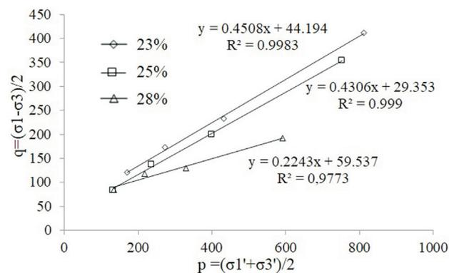
Figure 9. *p - q* diagrams for the three compaction moisture contents.
