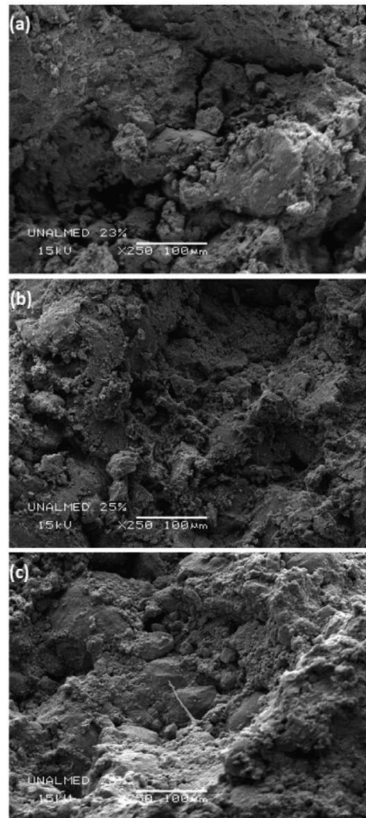
**Figure 2.** Images obtained by SEM for x250 magnification: (a) Image of compacted soil with 23 % moisture content; (b) Image of compacted soil with 25 % moisture content; (c) Image of compacted soil with 28 % moisture content.
