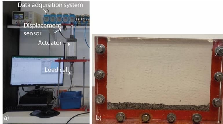
**Figure 2.** (a) Oedometric consolidometer apparatus for centrifuge models, (b) consolidated soil sample.
