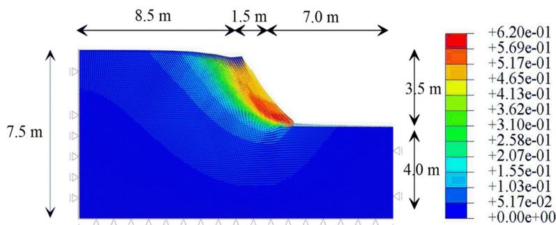
**Figure 5.** Example of an FEM model for boundary conditions and displacement results in the failure condition.
