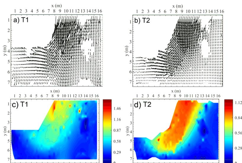
**Figure 7.** (a) Displacement vectors obtained with GeoPIV\_RG of model number one, (b) displacement vectors obtained with GeoPIV\_RG of model number two, (c) displacement resultants obtained with GeoPIV\_RG of model number one, (d) displacement resultants obtained with GeoPIV\_RG of model number two [adapted from Lozada et al. (2022)].
