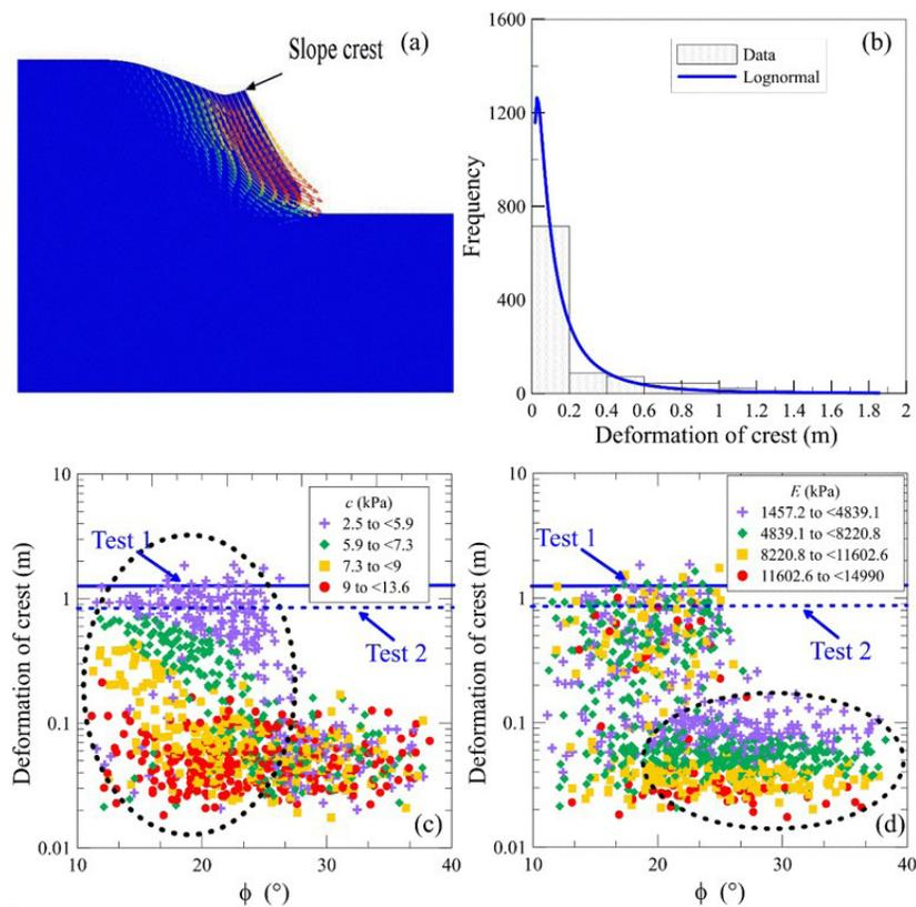
**Figure 12.** (a) Deformation vectors around of slope, (b) density curve and histogram of crest deformation, (c) and (d) deformation of crest versus variability of parameters.
