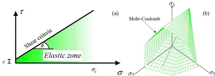
**Figure 4.** Scheme of the shear criteria to Mohr-Coulomb: (a)  $p$ - $q$  plane, (b)  $\pi$ -plane [adapted from Helwany (2007)].
