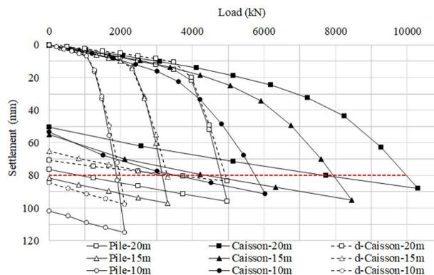
**Figure 3.** Load-settlement curves of the analyzed cases.
