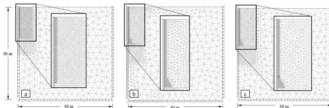
**Figure 2.** Numerically simulated axisymmetric models of: a) pile; b) pipe; c) defective caisson.
