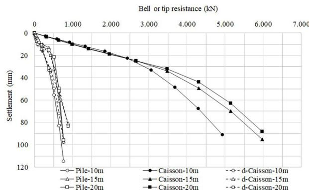
**Figure 5.** Tip resistance vs. settlement curves of the analyzed cases.
