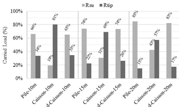
Figure 7. Skin friction and tip resistance of foundation types at different depths.
