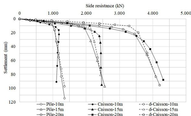
**Figure 4.** Skin friction resistance vs. settlement curves of the analyzed cases.
