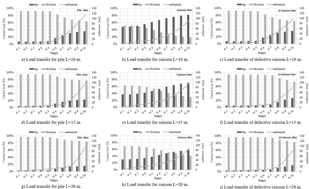
**Figure 6.** Load Transfer for piles, caisson and defective caisson for different shaft lengths.
