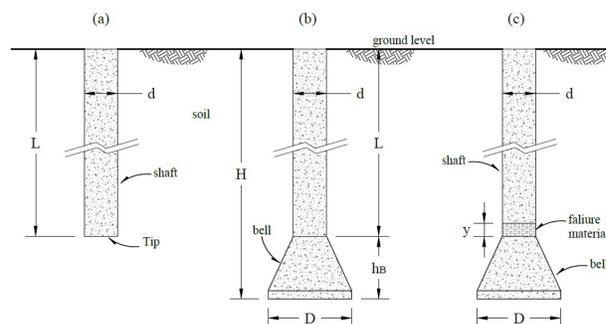
**Figure 1.** Schematic of the analyzed foundation types: a) pile (no bell); b) unimpaired caisson (with bell); c) defective caisson (with bell).
