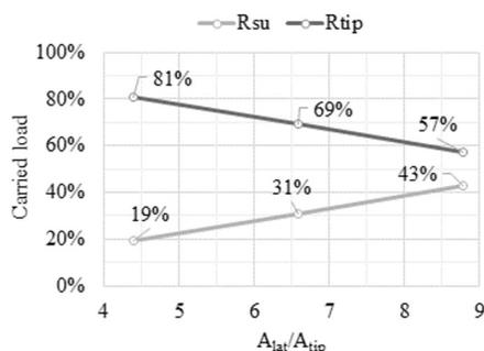
Figure 8. Load transfer to bell and shaft for different area ratios.
