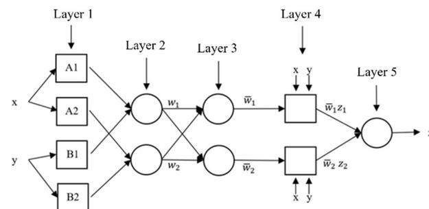
Figure 1. Diagram of an ANFIS neuro-fuzzy model (Jang, 1993).
