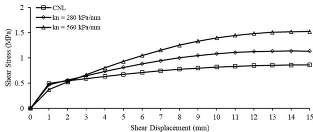
**Figure 6.** Effect of normal boundary stiffness on the shear stress ( $\sigma_{no} = 0.5$  MPa).
