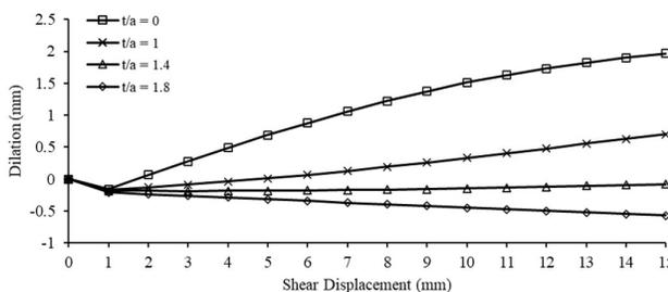
**Figure 5.** Effect of infill on the dilation ( $k_n = 425$  kPa/mm and  $\sigma_{n0} = 0.3$  MPa).
