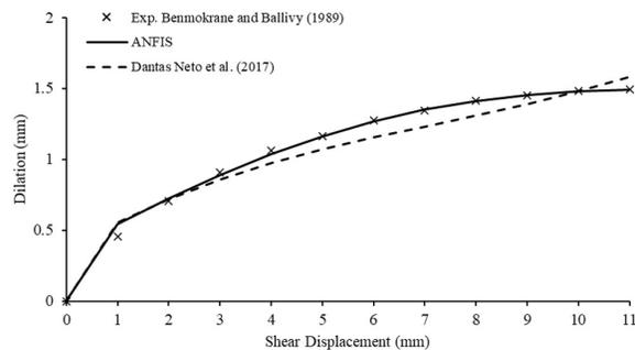
**Figure 12.** Comparison of experimental data for dilation of hard rocks and results from the *D1* ANFIS model and the ANN model proposed by Dantas Neto et al. (2017).
