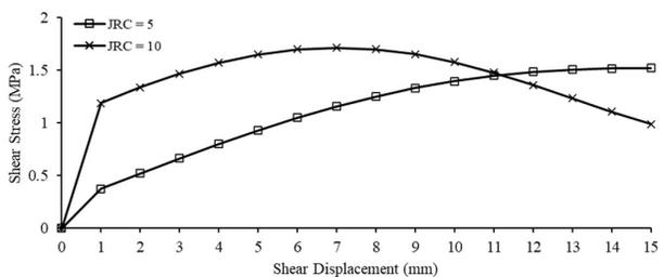
**Figure 9.** Effect of joint roughness on the shear stress ( $k_n = 560$  kPa/mm and  $\sigma_{no} = 0.5$  MPa).
