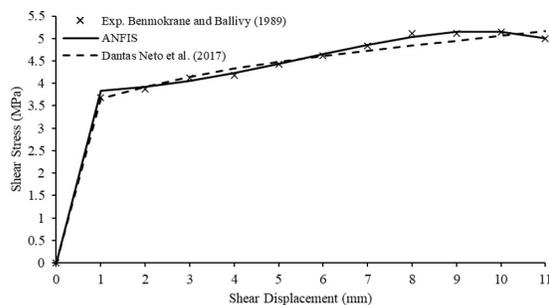
**Figure 13.** Comparison of experimental data for shear stress of hard rocks and results from the *S2* ANFIS model and the ANN model proposed by Dantas Neto et al. (2017).
