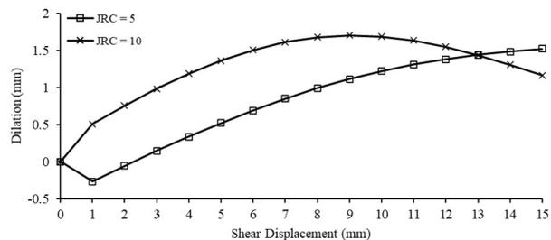
**Figure 4.** Effect of joint roughness on the dilation ( $k_n = 560$  kPa/mm and  $\sigma_{no} = 0.5$  MPa).
