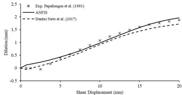
**Figure 10.** Comparison of experimental data for dilation of soft rocks and results from the *D1* ANFIS model and the ANN model proposed by Dantas Neto et al. (2017).
