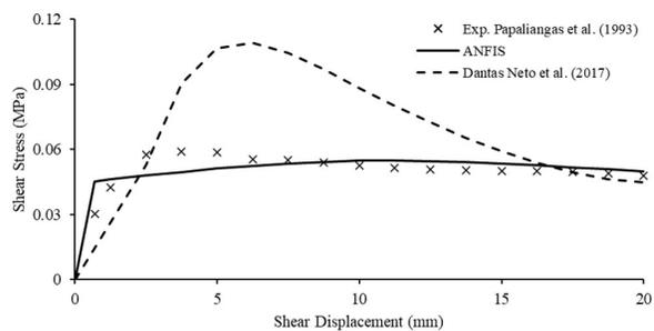
**Figure 11.** Comparison of experimental data for shear stress of soft rocks and results from the *S2* ANFIS model and the ANN model proposed by Dantas Neto et al. (2017).
