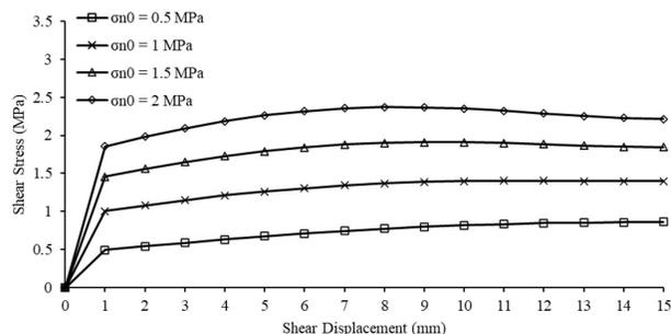
**Figure 7.** Effect of initial normal stress on the shear stress ( $k_n = 0$  kPa/mm).
