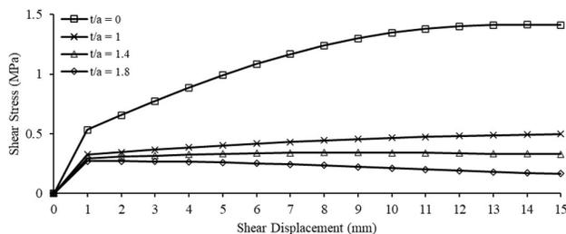
**Figure 8.** Effect of infill on the shear stress ( $k_n = 425$  kPa/mm and  $\sigma_{n0} = 0.6$  MPa).
