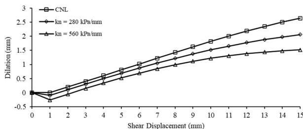
**Figure 2.** Effect of normal boundary stiffness on the dilation ( $\sigma_{no} = 0.5$  MPa).
