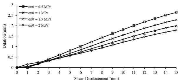
**Figure 3.** Effect of initial normal stress on the dilation ( $k_n = 0$  kPa/mm).
