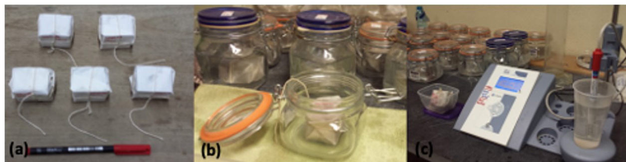
Figure 2. (a) sample packaging; (b) submersion for leaching test; (c) measurement of the leachate electrical conductivity.
