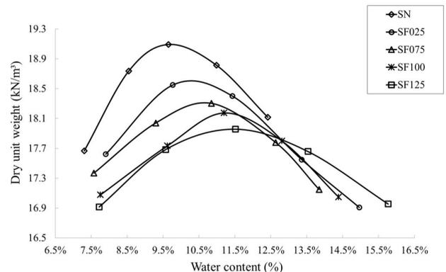
Figure 3. Compaction curves.
