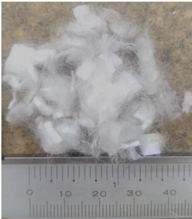
Figure 2. Polypropylene fibres.
