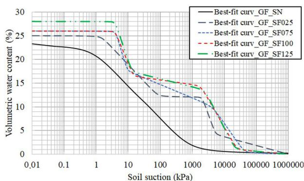
**Figure 10.** SWR curves with different fibre contents.
