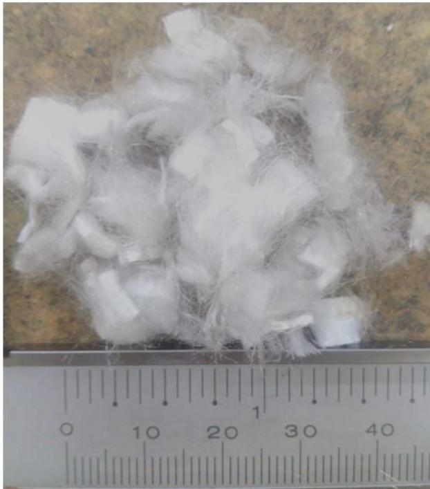
Figure 2. Polypropylene fibres.
