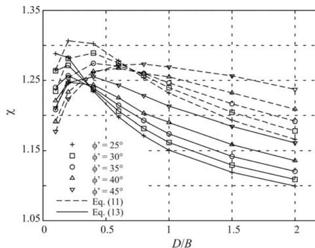
Figure 8 - Comparison between ratios  $\chi$  obtained from Eq. (11) for  $\gamma_1 = 20[FL^{-3}]$ , and Eq. (13), for  $\gamma_1 = 10[FL^{-3}]$ .
