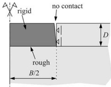
Figure 2 - Details of the footing-soil contact modelling.
