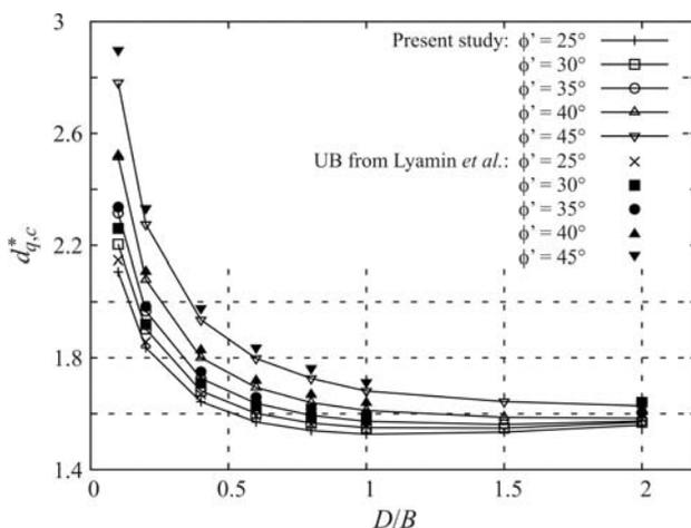
Figure 7 - Comparison between depth factor  $d_{q,c}^*$  (Eq. 12) obtained from the calculations of the present work and the upper-bound ones from Lyamin *et al.* (2007).
