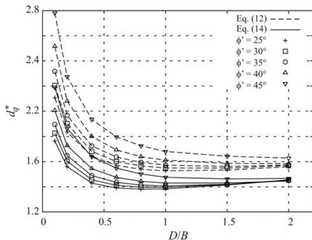
**Figure 9** - Comparison between depth factor  $d_q^*$  obtained in the present work using Eq. 12, for  $\gamma_1 = 20[FL^{-3}]$ , and Eq. (14), for  $\gamma_1 = 10[FL^{-3}]$ .
