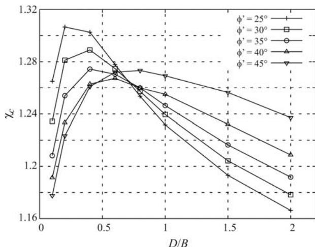
Figure 6 - Ratio  $\chi_c$  obtained from Eq. (11).
