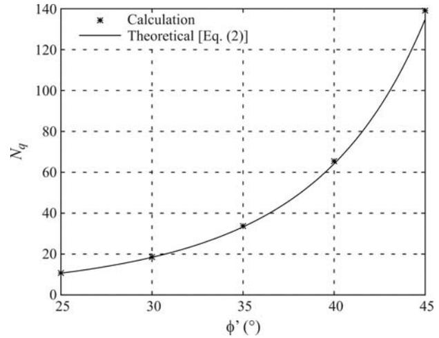
Figure 4 - Comparison between the values of the bearing capacity factor  $N_q$  obtained from limit analysis calculations and the theoretical ones.
