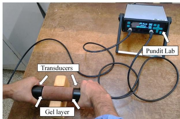
Figure 2. Ultrasonic test execution.
