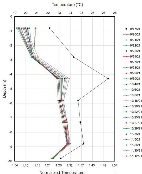
**Figure 13.** Underground temperature measurements and normalized temperature.
