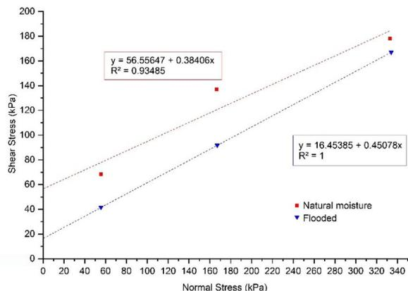
Figure 11. Shear strength envelopes for trench TR01.
