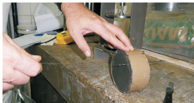
Figure 9 - Needle used to guide the introduction of a guitar string longitudinally into the sample.
