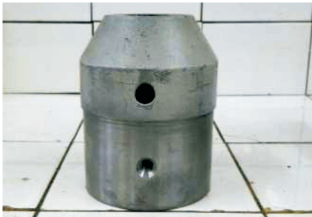
Figure 4 - Sampler head regularly used with thin wall brass sampler machined to be used with the thick wall plastic sampler.
