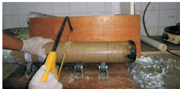
Figure 8 - Cutting the tube sampler with a band saw.
