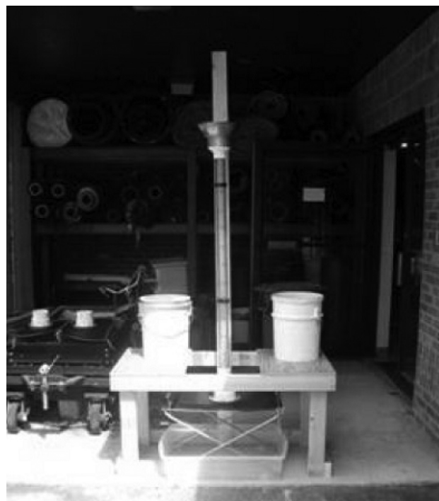
Figure 8 - Tests in geotextile closed according to GRI-GT15 (Geosynthetic Research Institute, 2009).
