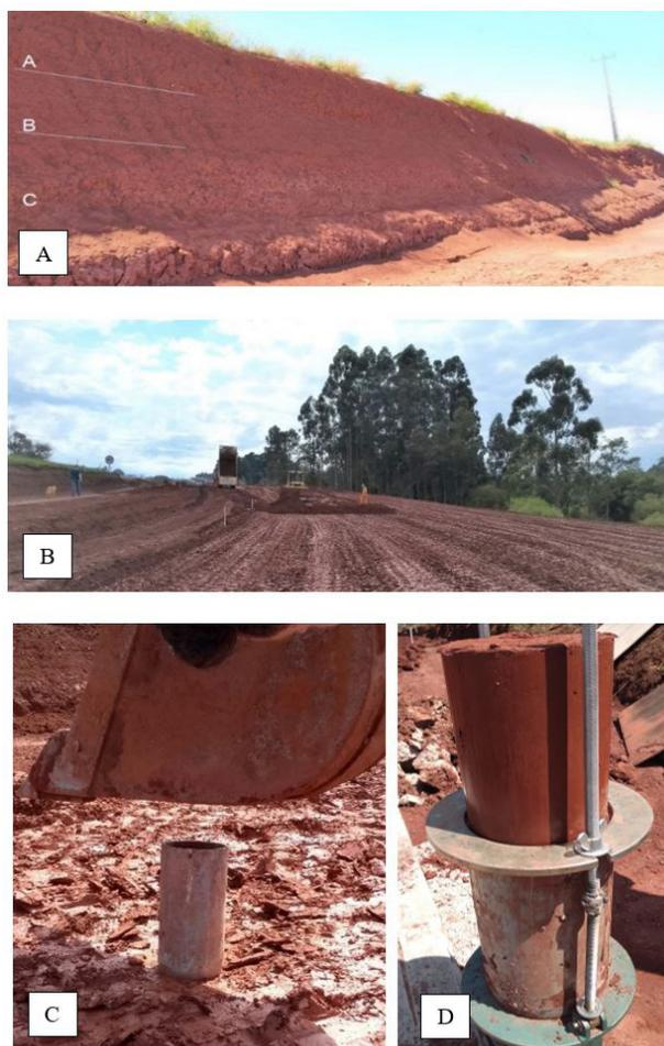
**Figure 1.** (A) Soil horizons at the Cruz Alta deposit, (B) location of the extraction of undisturbed soil sample, (C) sampler cylinder extraction procedure and (D) undisturbed soil sample.
