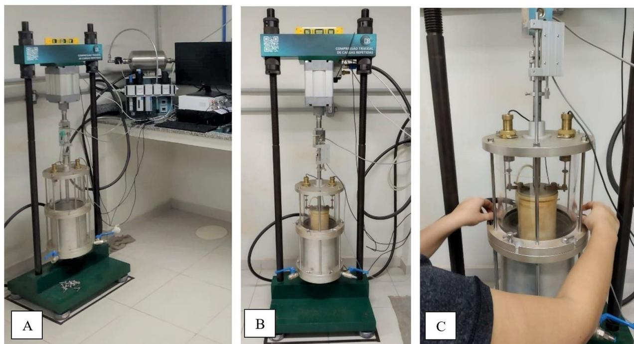
**Figure 2.** (A) Triaxial equipment of repeated loads, (B) soil sample being positioned on equipment, (C) detail of the two LVDTs inside the triaxial chamber.
