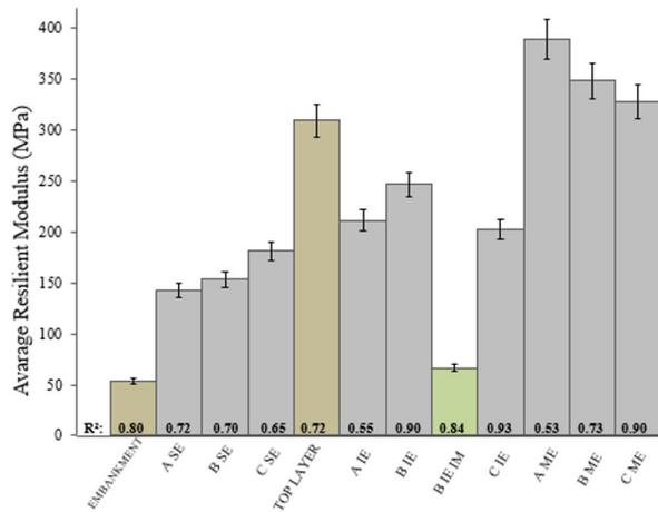
**Figure 7.** Average Resilient modulus determined by the compound model.
