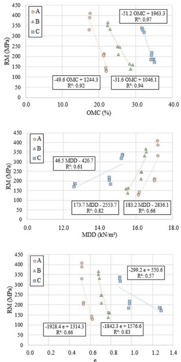
**Figure 8.** Correlations between the RM and the physical indexes for the samples analyzed with compound model.
