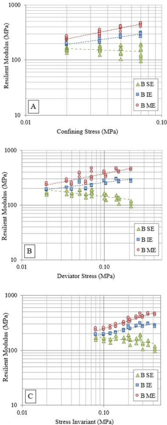
**Figure 5.** RM behavior for horizon B at three compaction energy levels, based on the (A) Biarez, (B) Svenson and (C) stress invariant models.
