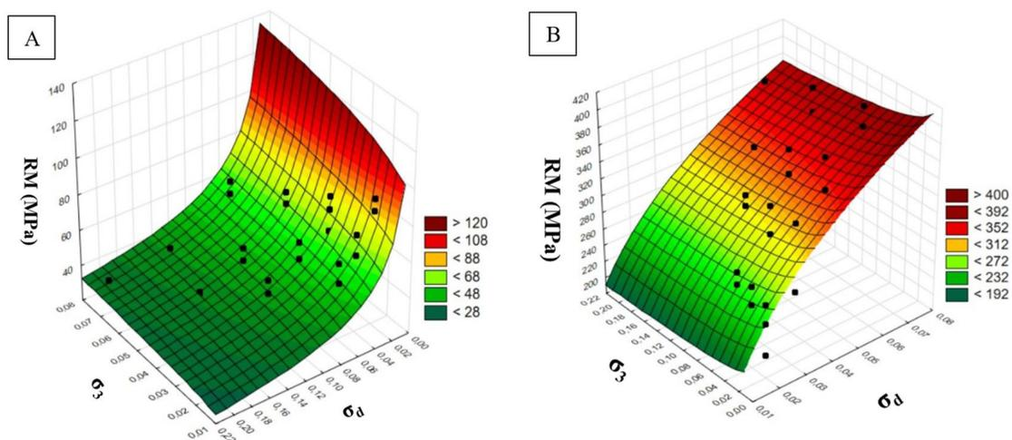
**Figure 6.** Three-dimensional graph of the undisturbed samples from the (A) interior of embankment and the (B) top layer, using the compound model.
