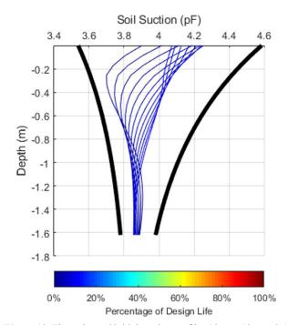
**Figure 12.** The estimated initial suction profiles (time = 12 months) for TX 48-1068 SMP section.
