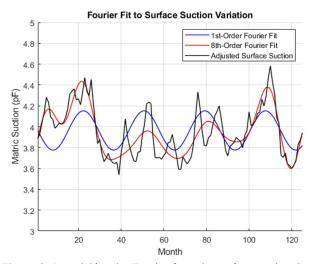
**Figure 9.** 1<sup>st</sup> and 8<sup>th</sup> order Fourier fit to the surface suction data for the TX 48-1068 section for the date range 3/1987 to 9/1997.
