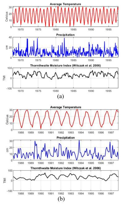
**Figure 2.** Monthly average temperature and rainfall data for NOAA weather station USC00416794 with the calculated yearly *TMI* (Witczak et al., 2006) between (a) 9/1967 and 9/1997 and (b) 3/1987 and 9/1997.
