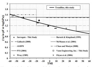
Figure 5. Limits of the potential change in suction at the surface vs. *TMI* with literature values (Vann & Houston, 2021).
