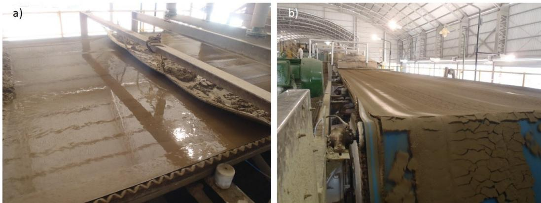
**Figure 2.** Vacuum belt filter at Casposo Mine. (a) Tailings being fed to the filter band; (b) Tailings at filter output.
